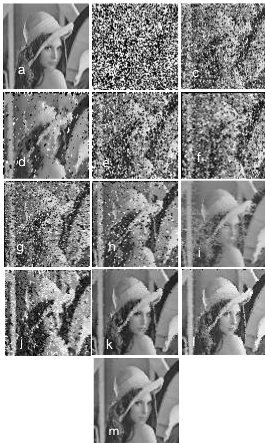
Fig.8 Performance of Test image: Lena (a) Noise free images, (b) image corrupted by 70% impulse noise, (c) images restored by MF, (d) images restored by WMF, (e) images restored by CWMF, (f) images restored by TSMF, (g) images restored by NID, (h) images restored by MDBSMF, (i) images restored by DBSMF, (j) images restored by NFT, (k) images restored by MDBUTMF, (l) images restored by NBPPFT and (m) image restored by proposed filter
